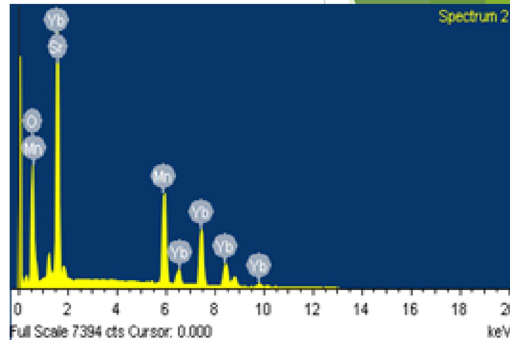
XRD and EDAX of  $\text{Yb}_{0.9}\text{Sr}_{0.1}\text{MnO}_3$
